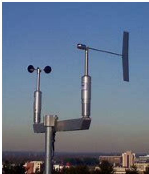
Figure 4 - The installation of a wind vanes will help control of the smoke control system
